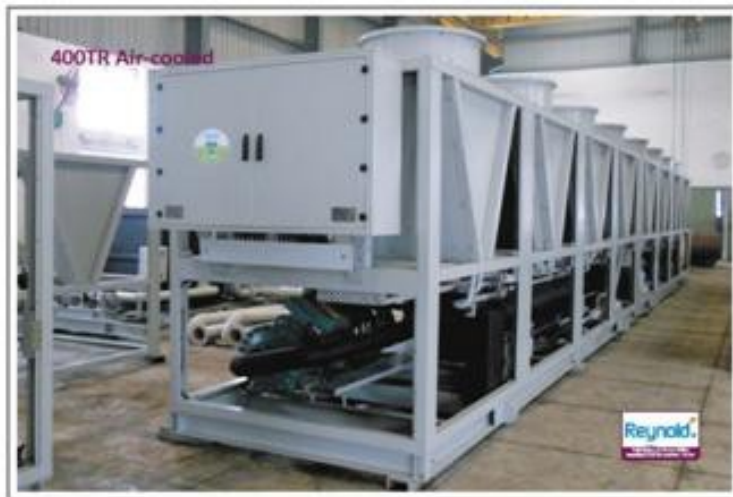
400 TR, Air Cooled for process cooling
