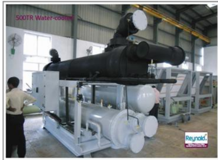
500 TR, Water Cooled for process cooling
